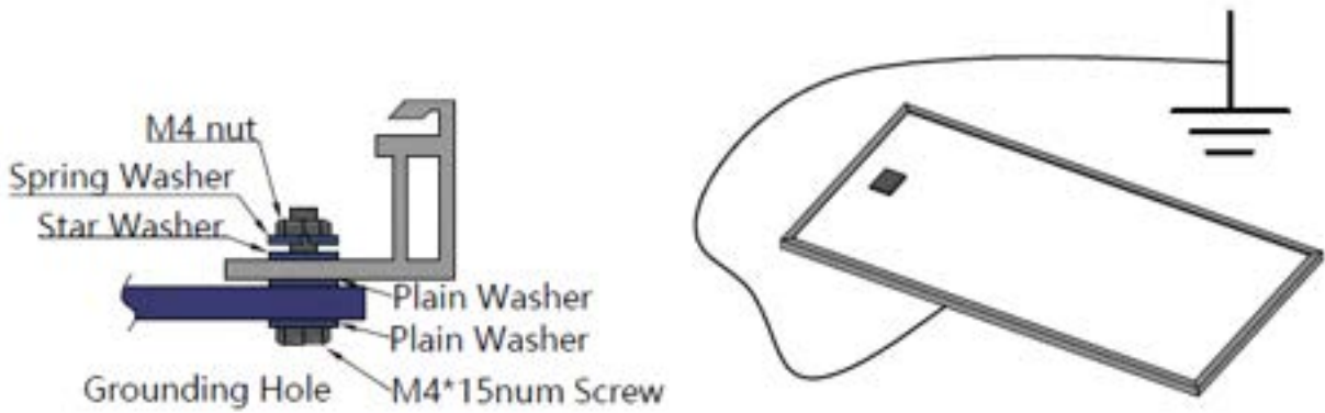
Figure 9: Ground installation of PV modules
